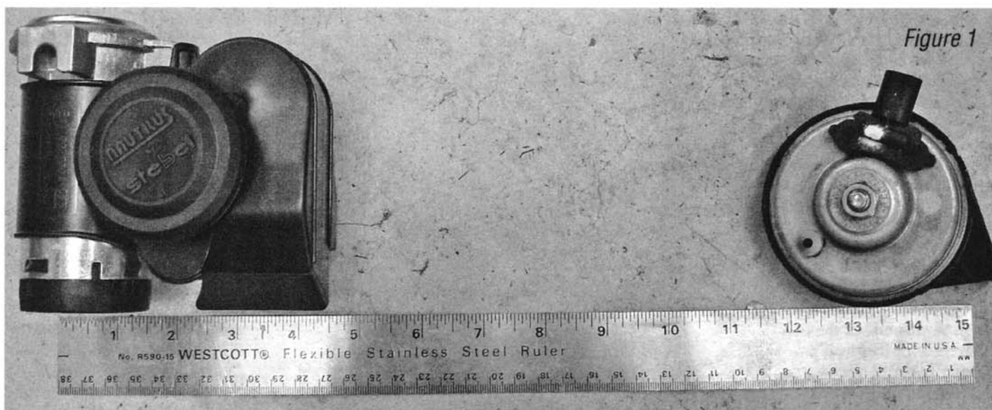
The Stebel Compact Nautilus Air Horn on the left is only about an inch wider than the stock Bosch unit on the right.
